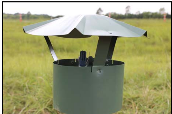
f) Mounted Temp/Humidity Instrumentation
