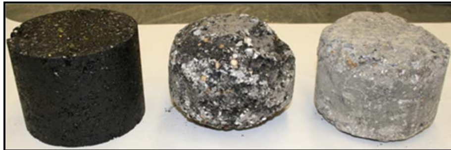
Figure 4.15. Example Asphalt Concrete Cantabro Specimens (L: Untested, M: High M_L , R: Low M_L )
