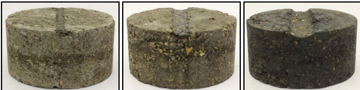
a) Cement SCB b) Cement-Emulsion MCB c) Emulsion SCB
