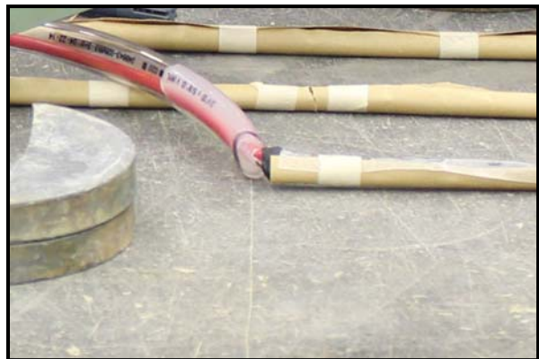
f) Flex Tubing and Aqua Seal™ Junction
