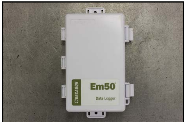
b) Decagon Em50 Data Logger for GS3 Sensors
