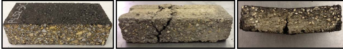
a) Untested Asphalt Concrete b) Tested CIR – Cement SCB c) Tested CIR – Emulsion SCB
