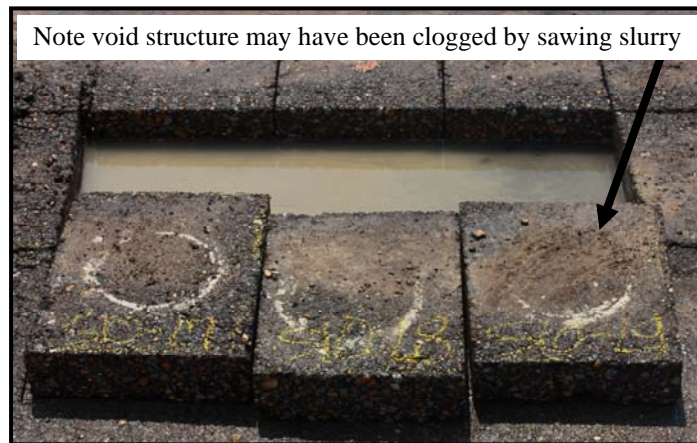
Figure 3.10. MSP-L L Test Slabs Cut from Parking Lot
