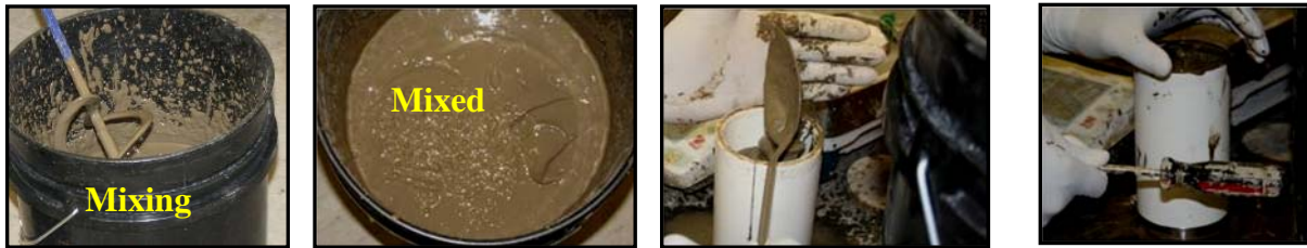
Figure 5.1. LC-VHMS Specimen Preparation-Portland vs. Slag/Portland Cement
