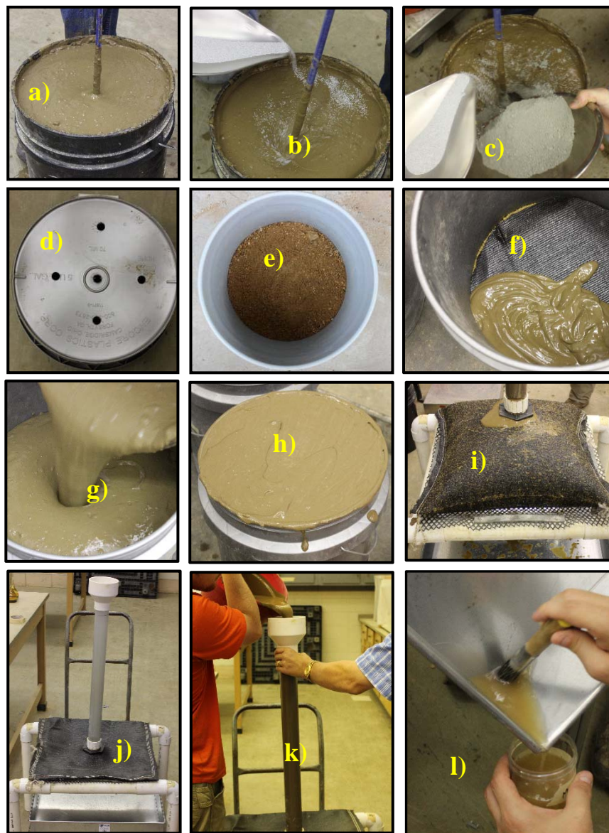
Figure 8.1. Vegetation Experiment Specimen Preparation: Buckets & Geotextile Pillows
