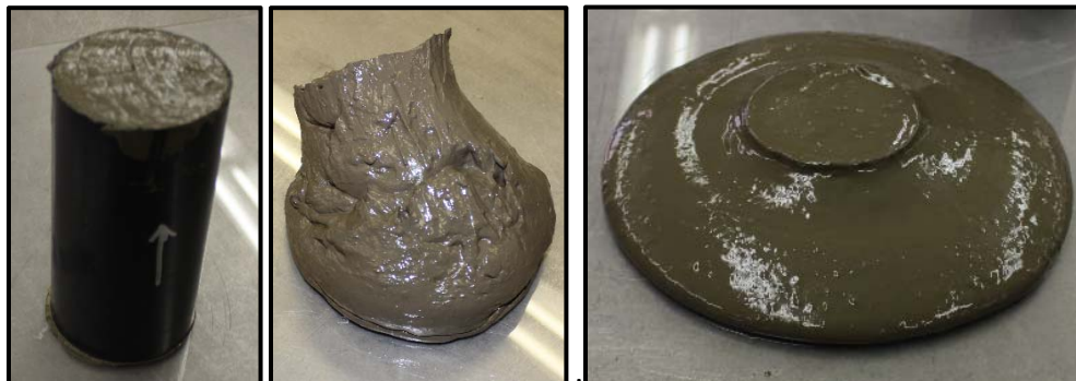
Figure 7.1. ASTM D 6103 Testing
