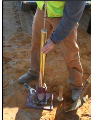
Figure 5.16. Specimen Compaction as per PM-P Approach
