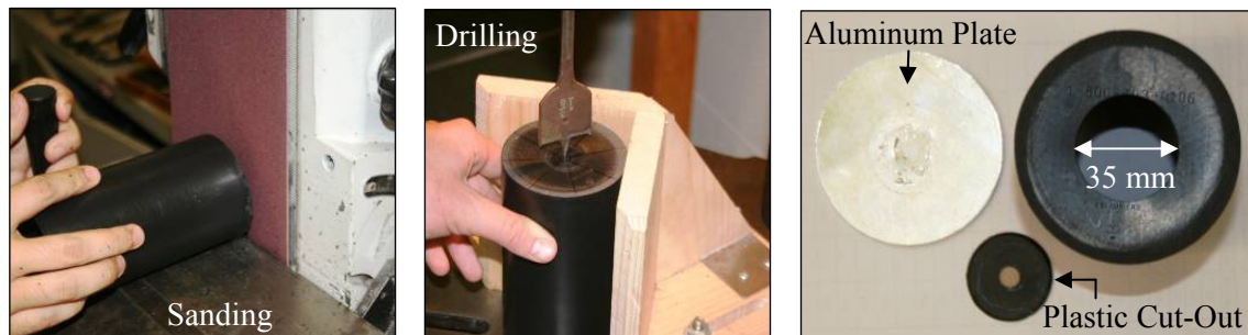
Figure 5.1. 76.2 by 152.4 mm Plastic Mold Modifications
