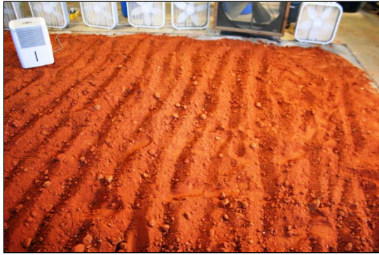
(a) Air Drying of Soil
