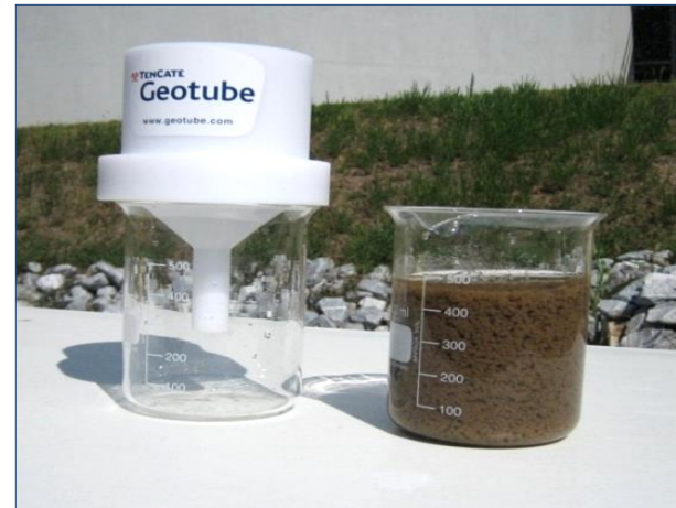
Rapid Dewatering Test (RDT)
