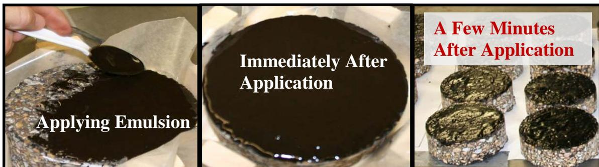
Figure 4.1. Applying Emulsion to Cores
