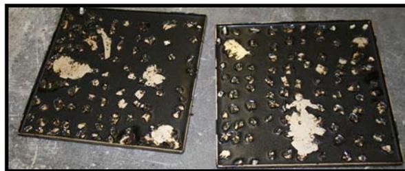
**Figure 8.1. *Vialit* Specification Trays After Testing**
