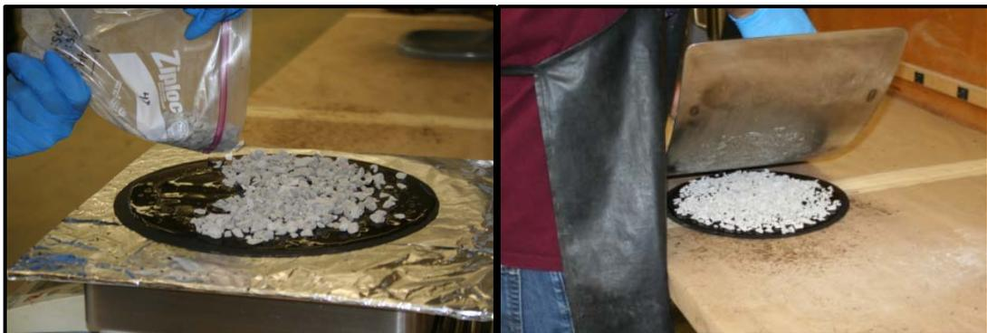
c) *Aggregate Spreading*                      d) *Aggregate Compaction*
