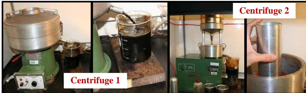
**Figure 4.6. Asphalt Extraction Equipment**
