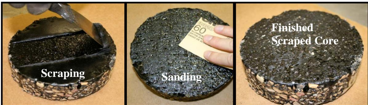
**Figure 4.3. Scraping Emulsion Treated Core**
