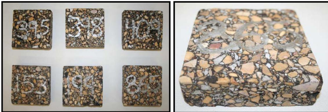
**Figure 3.3. Blocks Sawn From Field Aged Pavement for  $G_{mb}$  Measurement**
