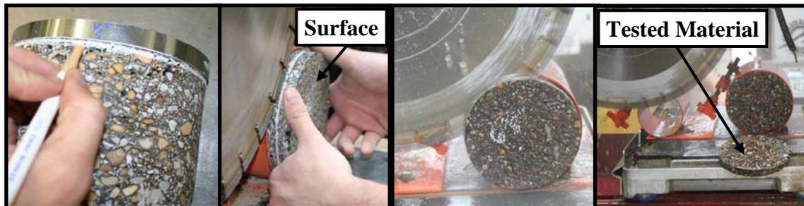
Figure 4.5. Slicing Cores for Viscosity Testing-Untreated Core Shown
