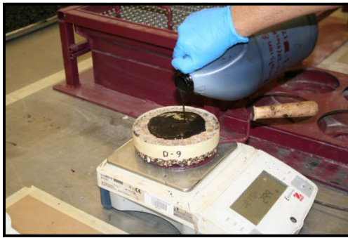
a) Emulsion Poured on Core
