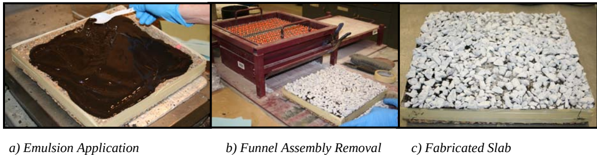
Figure 4.11. Specimen Fabrication Procedure - Slabs
