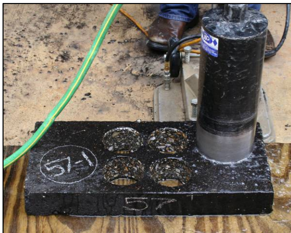
(c) 152.4 mm Coring Process
