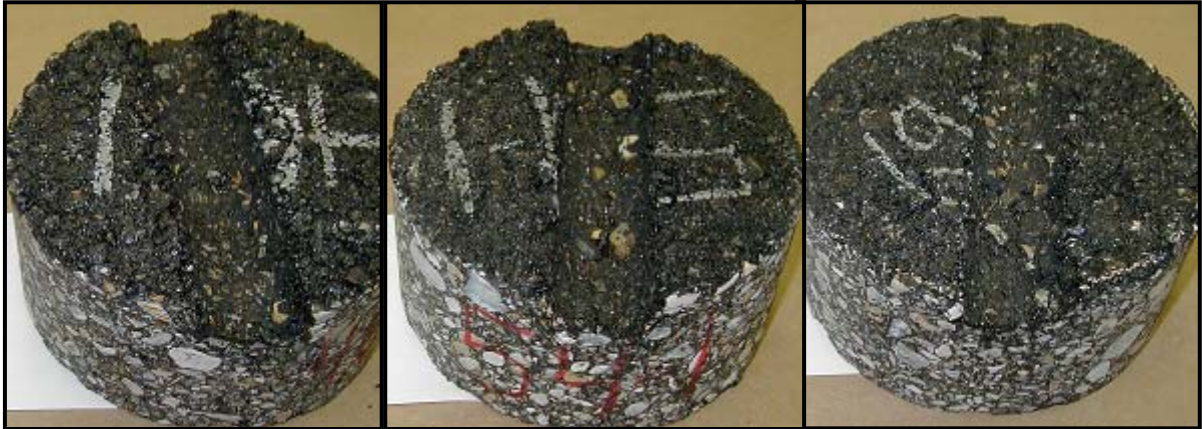
Figure H-20. APA Slab Specimens Indicating Uniform Deformation
