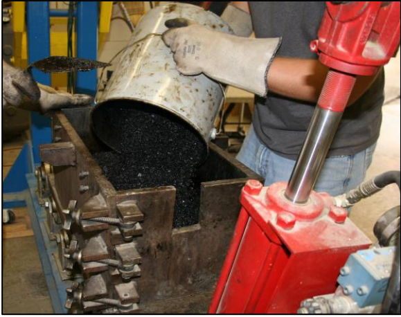
(a) Loading Mix into LAC Compaction Mold
