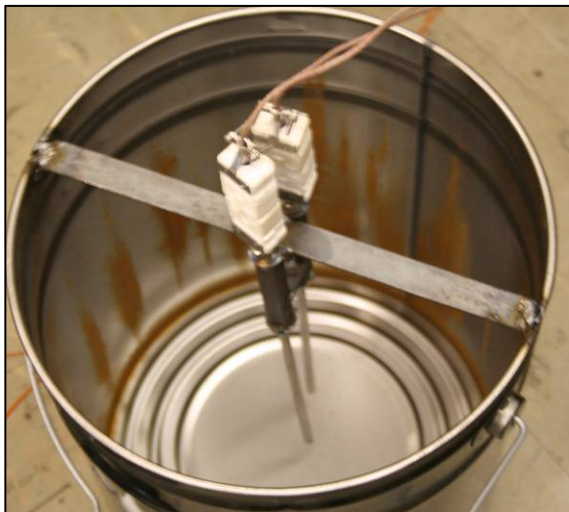
(c) Probe Thermocouples and Fixtures
