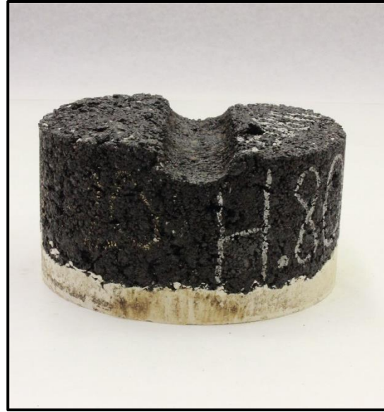
b.) APA Tested Specimen
