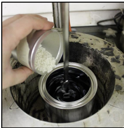
Figure 2.3. Sasobit® Being Mixed into Binder
