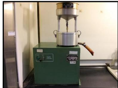
*c) ASTM D1856 centrifuge*
