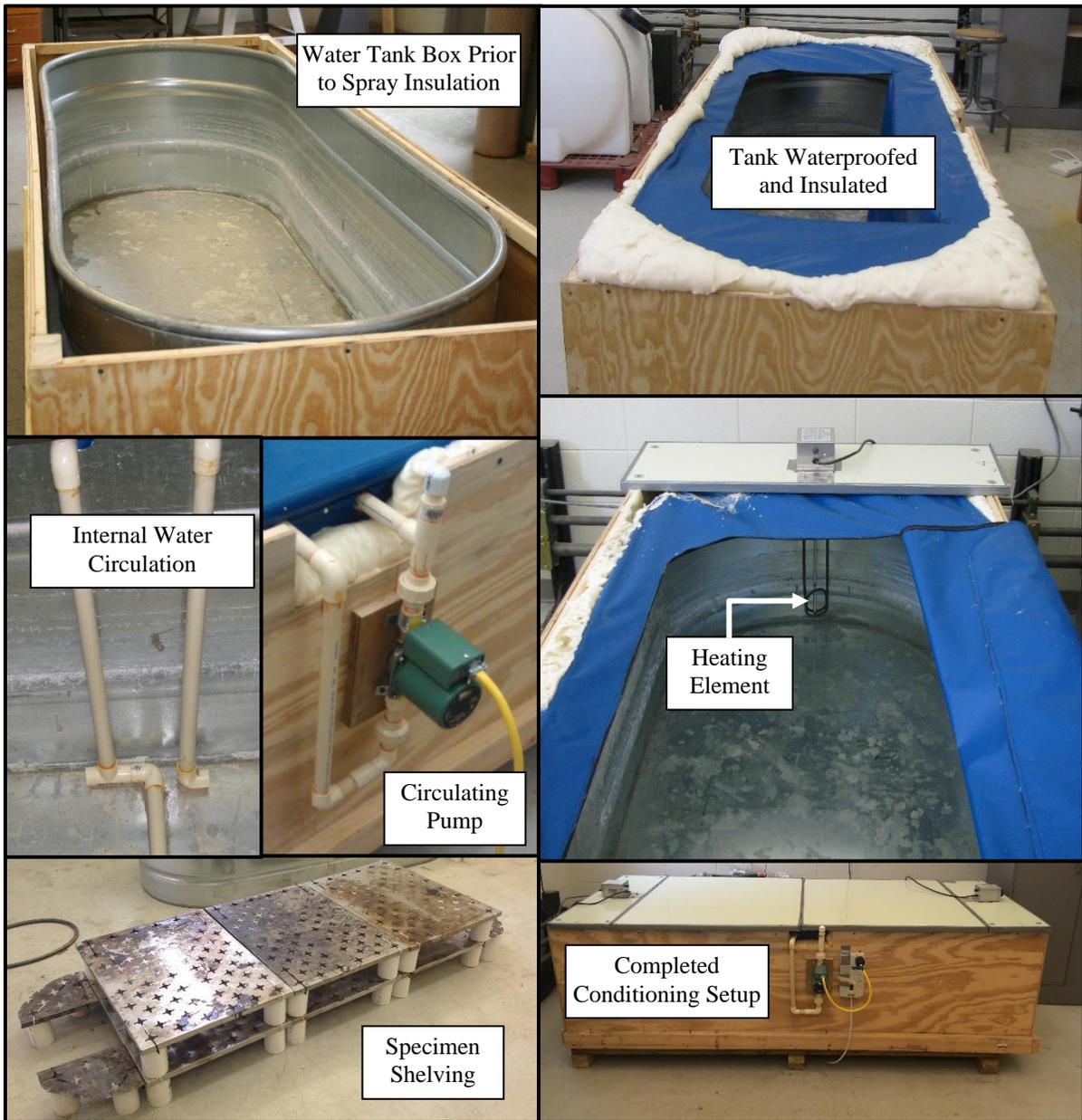
**Figure 3.12. Water Conditioning Tank**
