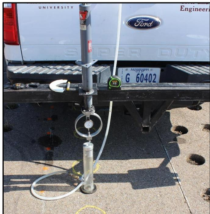
b) MSP Field Testing Vehicle Support Frame
