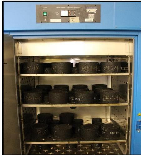
**Figure 3.3. Example Oven Conditioning Photograph**
