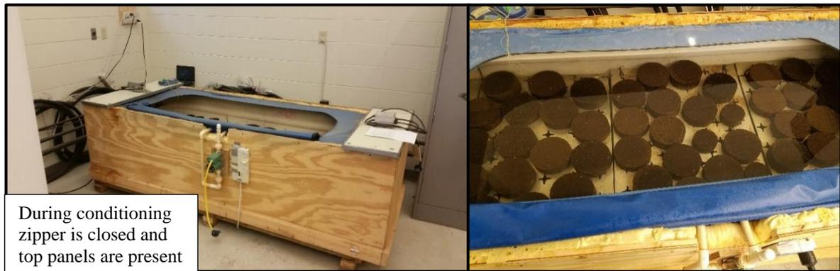
**Figure 3.4. Example of Water Conditioning.**
