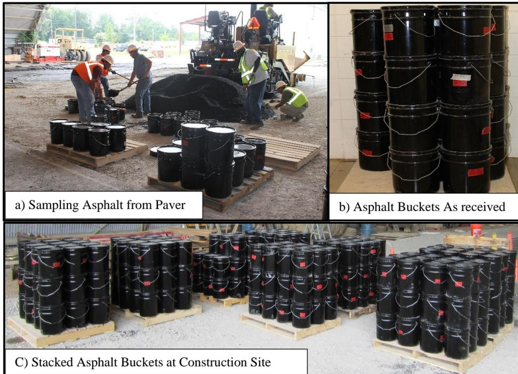
**Figure 3.1. Stacked Asphalt Buckets Prior to Testing**
