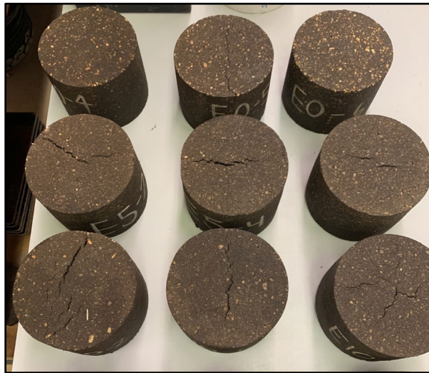
Figure 3.1. Visual Damage to Sand Asphalt During CP7 Conditioning
