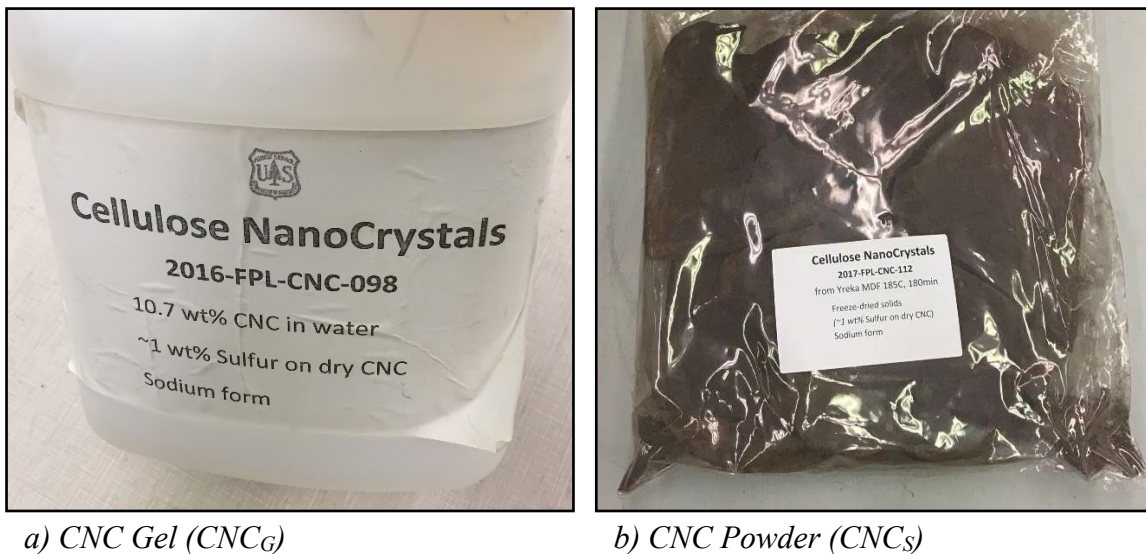
Figure 2.1. Photos of CNC Materials As Supplied by USDA-FPL
