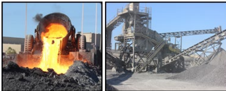
Figure 3.1. Steel Slag Manufacturing Process
