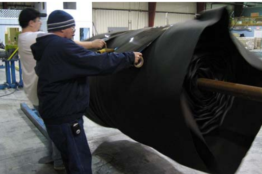
(g) Rolling Geotextile Tube Onto Pipe
