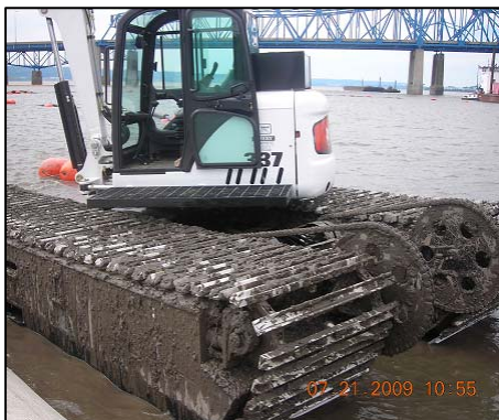
Figure 3.32. Amphibious Trackhoe Used at Peoria Island
