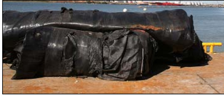
Figure 3.7. Geotextile and Anchor Tubes Used at Matagorda Ship Channel
