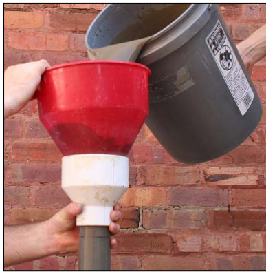
(c) Slurry Entering Tube
