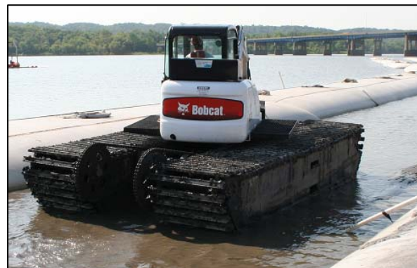
Figure 3.32. Amphibious Trackhoe Used at Peoria Island
