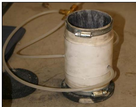
*Figure 3.13. Mold With Thin Membrane Inserted*
