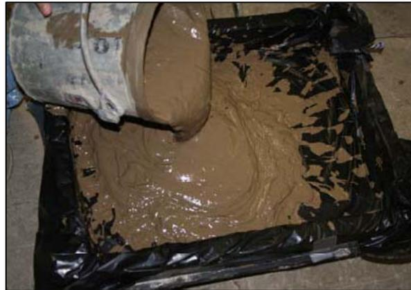
(b) Pouring Stabilized Slurry Into Mold
