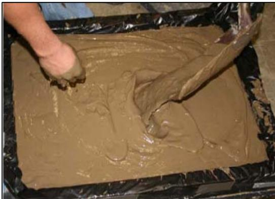
(c) Shoveling Stabilized Slurry Into Mold
