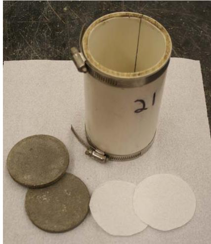
**Figure 3.12. Unconfined Compression (UC) Specimen Molds**
