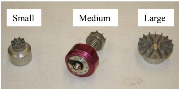
(c) Pocket Vane Shear Set (Shear)
