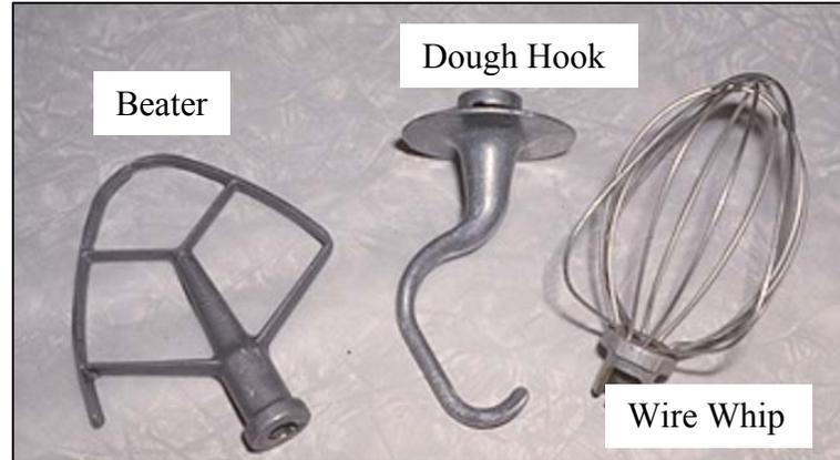
**Figure 2.1. Attachments for Industrial Mixers**
