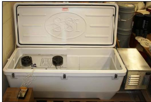
**Figure 3.26. Curing Chamber Used During Select SAC Testing**
