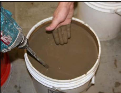
(e) *Soil Slurry Prior to Aging*
