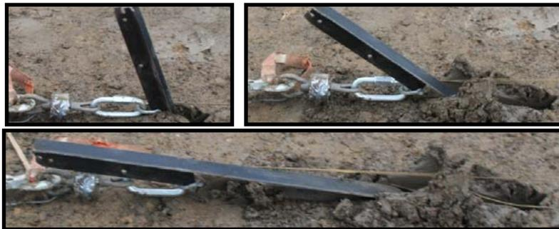
**Figure 4.9. Star Picket (0.3 m) Anchor During Testing**
