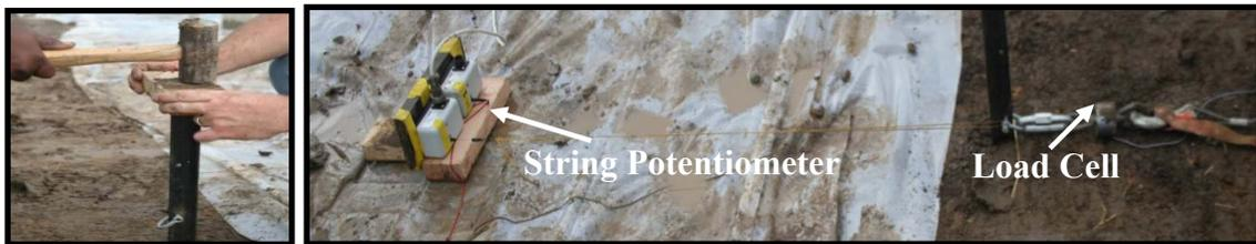
**Figure 4.8. Installation of 0.3 m Star Picket**
