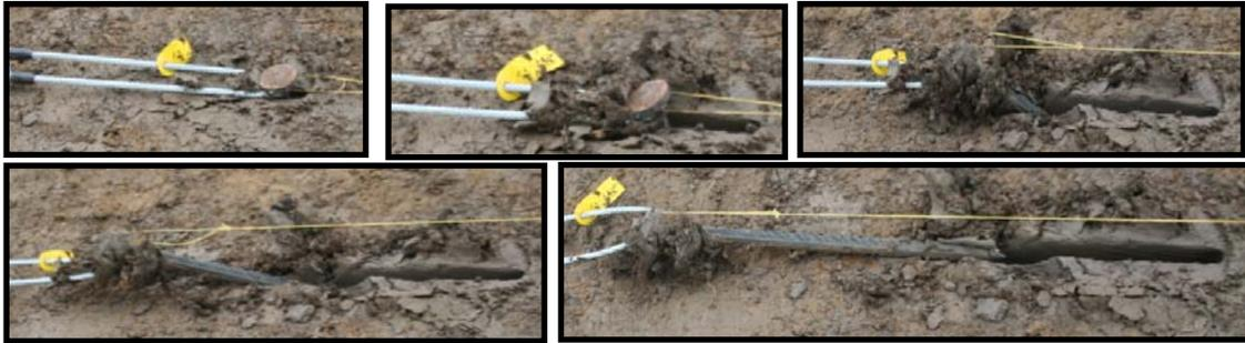
**Figure 4.7. Mobi Stake (0.6 m) Anchor During Testing**
