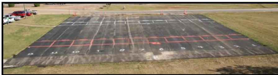
**Figure 11. Hot-Mixed and Warm Compacted Parking Lot Test Sections**
