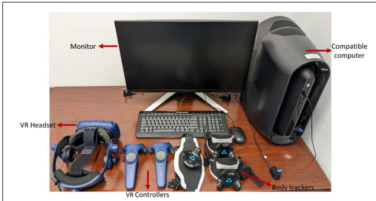
Figure 2. Computer, VR headset, controllers, and body trackers for the training system
