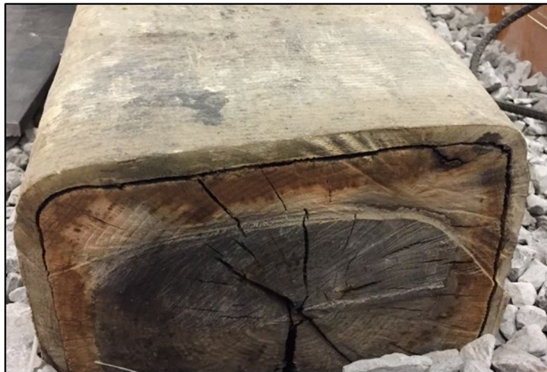
Figure 4.1. Example GFRP-wrapped wooden railroad tie cross section
