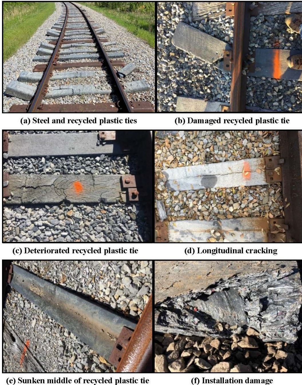
Figure 3.2. RPL and composite tie implementation issues
