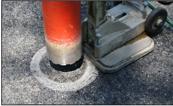
(a) Coring of FWD Test Location
