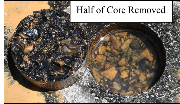
(b) Example of Stripped Core
